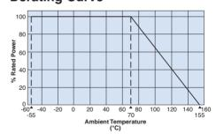
For resistors operated at an ambient temperature of 70°C or above, the power rating shall be derated in accordance with the above derating curve.
