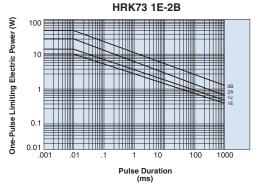
The maximum applicable voltage is equal to the max. overload voltage. Please ask us about the resistance characteristic of continuous applied pulse.
