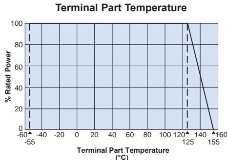
For resistors operated terminal part temperature of described for each size or above, a power rating shall be derated in accordance with the derating curve. Please refer to "Introduction of the derating curve based on the terminal part temperature" in the beginning of our catalog before use.
