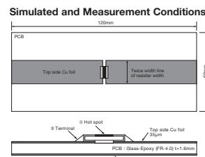
Temperature rise is simulated and measured under our conditions.
