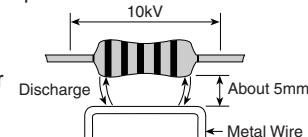
For example: In the figure, a metal wire is placed less than 5mm away from the resistor body, there is such a case that causes an electric discharge by a surge load 10kV and then destroys the outer coating.
