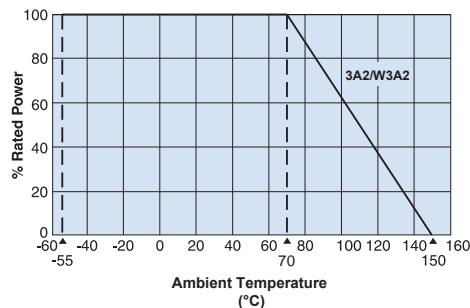
For resistors operated at an ambient temperature of 70°C or above, the power rating shall be derated in accordance with the above derating curve.
