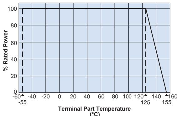
For resistors operated at a terminal part temperature of described for each size or above, a power rating shall be derated in accordance with the above derating curve.
