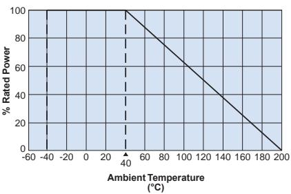
For resistors operated at an ambient temperature of 40°C or above, a power rating shall be derated in accordance with the derating curve.
