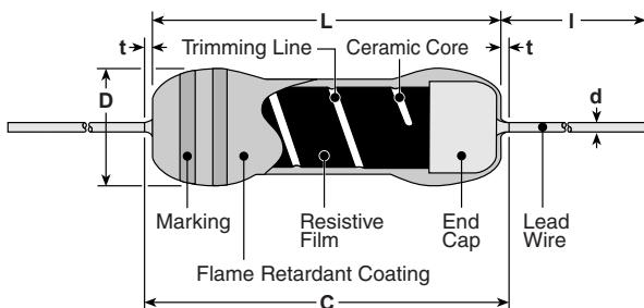
\* Lead length changes depending on taping and forming.
