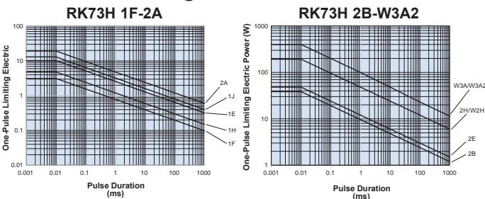
The maximum applicable voltage is equal to the max. overload voltage. Please ask us about the resistance characteristic of continuous applied pulse. The pulse endurance values are not assured values, so be sure to check the products on actual equipment when you use them.
