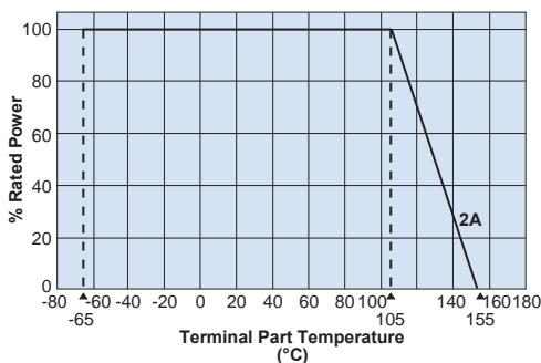
For resistors operated at an ambient temperature of 105°C or above, a power rating shall be derated in accordance with the above derating curve.
