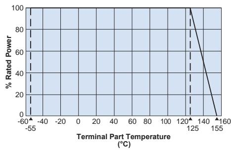
For resistors operated terminal temperature of described for each size or above, a power rating shall be derated in accordance with the derating curve. Please refer to "Introduction of the derating curve based on the terminal part temperature" in the beginning of our catalog before use.
