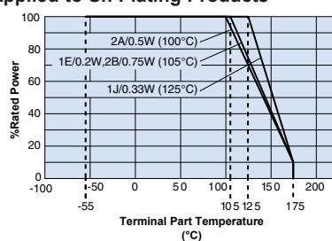
When the terminal part temperature of the resistor exceeds the rated terminal part temperature shown above, the power shall be derated according to the derating curve.
