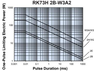
Please ask us about the resistance characteristic of continuous applied pulse. Please calculate One-Pulse Limiting Electric Power using upper limit of resistance (50mΩ or 100mΩ) for applied current. The pulse endurance values are not assured values, so be sure to check the products on actual equipment when you use them.
