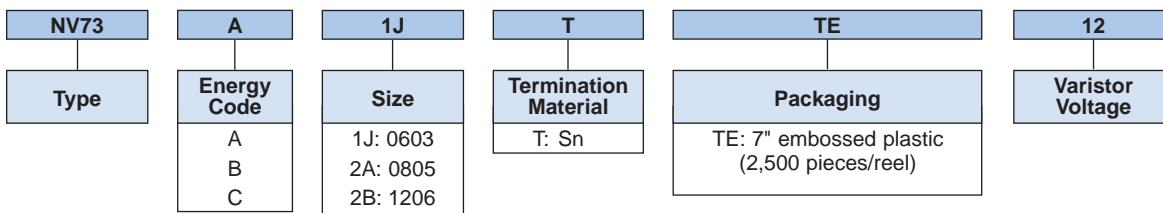
The terminal surface material lead free is standard.
