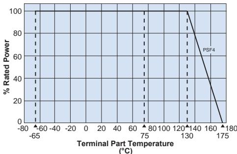
When the terminal part temperature of the resistor exceeds the rated terminal part temperature shown, the power shall be derated according to the derating curve.
