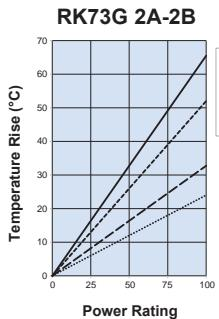
Regarding the temperature rise, the value of the temperature varies per conditions and board for use since the temperature is measured under our measuring conditions.
