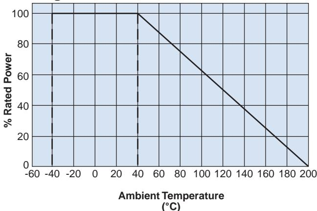
For resistors operated at an ambient temperature of 40°C or higher, the power rating shall be derated in accordance with this derating curve.
