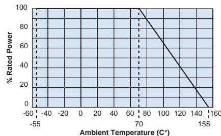
For resistors operated at an ambient temperature of 70°C or above, a power rating shall be derated in accordance with the derating curve.
