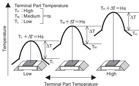
The temperature of the resistor will increase the same  $\Delta T$  from the standard terminal part temperature regardless of the ambient temperature when the same power is applied. This is because there is hardly any heat dissipation from the resistor surface to the ambient air.
