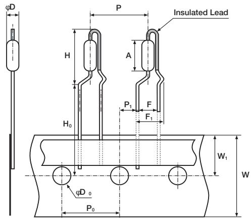
**VTP Radial Taping**
