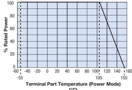
For resistors operated at an ambient temperature of  $85^\circ\text{C}$  or above, a power rating shall be derated in accordance with the above derating curve.
