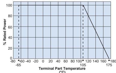
For resistors operated terminal temperature of described for each size or above, a power rating shall be derated in accordance with the derating curve above.
