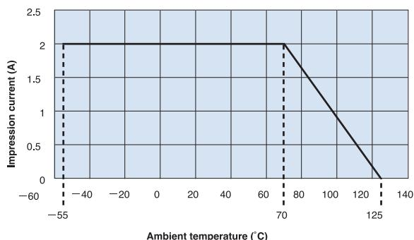
For terminals operated at an ambient temperature of 70°C or higher, the current shall be derated in accordance with the above derated curve.
