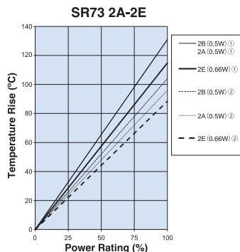
Regarding the temperature rise, the value of the temperature varies per conditions and board for use since the temperature is measured under our measuring conditions.
