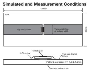
Temperature rise is simulated and measured under our conditions.
