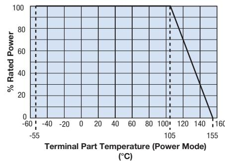
For resistors operated at an ambient temperature of 85°C or above, a power rating shall be derated in accordance with the above derating curve.
