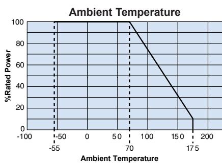
For resistors operated at an ambient temperature of 70°C or above, a power rating shall be derated in accordance with the derating curve.
