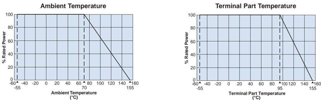
For resistors operated at an ambient temperature of 70°C or above, a power rating shall be derated in accordance with the above derating curve.
