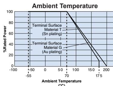
For resistors operated at an ambient temperature of 70°C or above, a power rating shall be derated in accordance with the derating curve.
