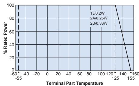
For resistors operated at a terminal part temperature of described for each size or above, a power rating shall be derated in accordance with the derating curve. Please refer to "Introduction of the derating curve based on the terminal part temperature" in the beginning of our catalog before use. \*1 If you want to use the rated power of \*1, please use the derating curve based on the terminal part temperature on the right hand side.
