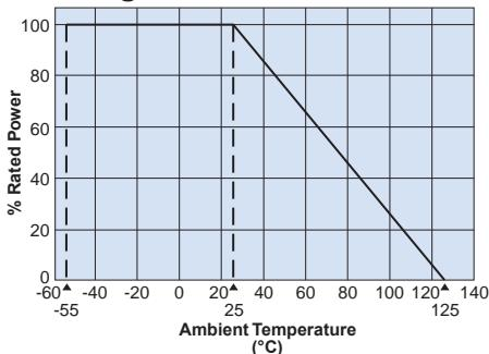
For resistors operated at an ambient temperature of 25°C or above, a power rating shall be derated in accordance with the above derating curve.
