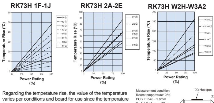
Regarding the temperature rise, the value of the temperature varies per conditions and board for use since the temperature is measured under our measuring conditions.
