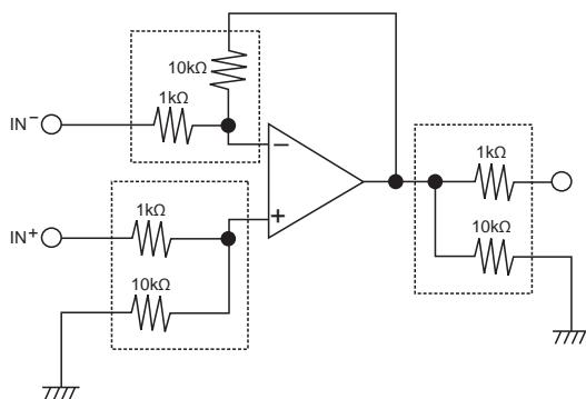
**merit of thin film resistor networks**
