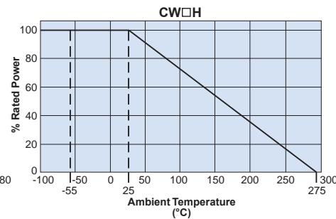
For resistors operated at an ambient temperature of 25°C or above, a power rating shall be derated in accordance with the above derating curve.
