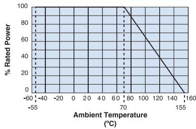
For resistors operated at an ambient temperature of  $70^{\circ}\text{C}$  or above, a power rating shall be derated in accordance with the derating curve.
