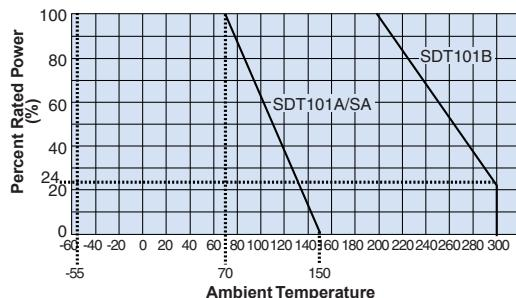
For sensors operated at an ambient temperature or above, a power rating shall be derated in accordance with the above derating curve.
