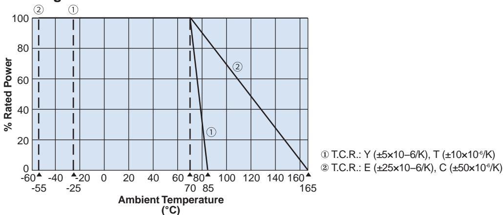
For resistors operated at an ambient temperature of 70 $^{\circ}$ C or above, a power rating shall be derated in accordance with the above derating curve.
