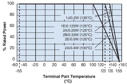
For resistors operated at a terminal part temperature of described for each size or above, a power rating shall be derated in accordance with the derating curve.
