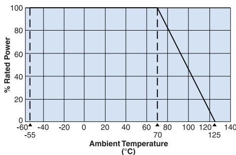
For sensors operated at an ambient temperature of 70 $^{\circ}$ C or above, a power rating shall be derated in accordance with the above derating curve.
