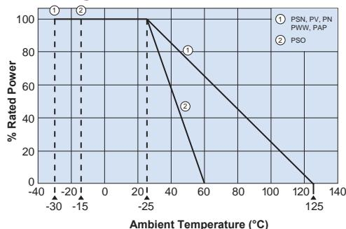
For resistors operated at an ambient temperature of 25°C or above, a power rating shall be rated in accordance with the above derating table.
