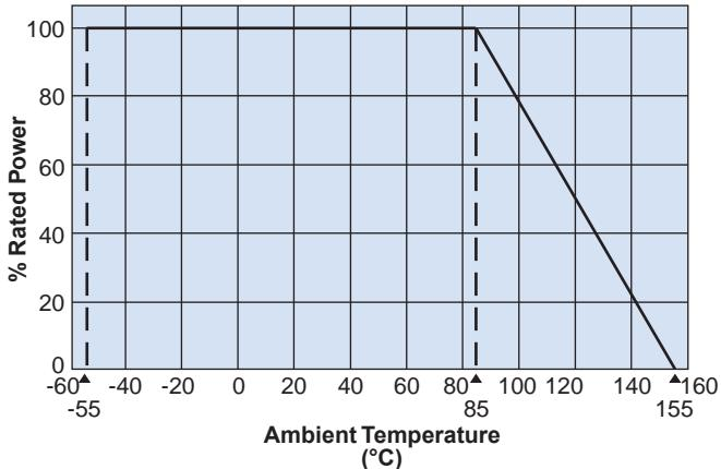
For resistors operated at an ambient temperature of 85°C or above, a power rating shall be derated in accordance with the derating curve.
