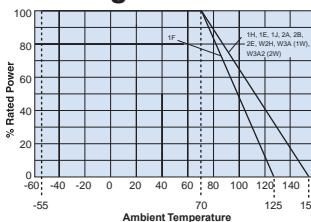
For resistors operated at an ambient temperature of 70°C or higher, the power shall be derated in accordance with the above derating curve.
