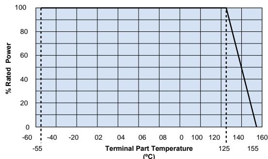
For resistors operated terminal part temperature of described for each size or above, a power rating shall be derated in accordance with the derating curve. Please refer to "Introduction of the derating curve based on the terminal part temperature" in the beginning of our catalog before use.
