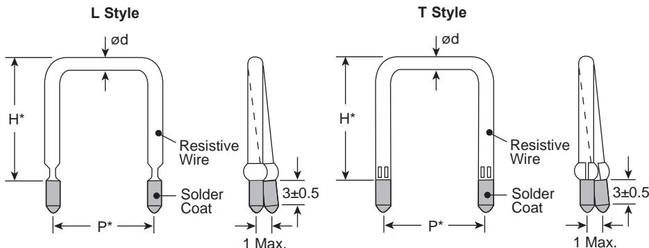
\* Please consult with factory about dimensions "P" and "H". T style is applied for the diameter of  $\varnothing$  2.3 or above
