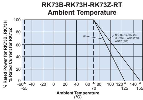
For resistors operated at an ambient temperature of 70°C or higher, the power (for RK73B, RK73H) or a current rating (for RK73Z) shall be derated in accordance with the above derating curve.
