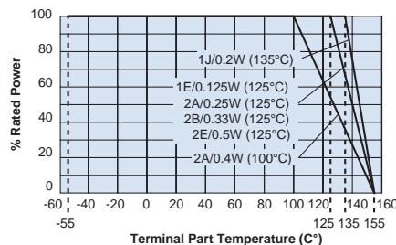
For resistors operated at a terminal part temperature of described for each size or above, a power rating shall be derated in accordance with the derating curve.
