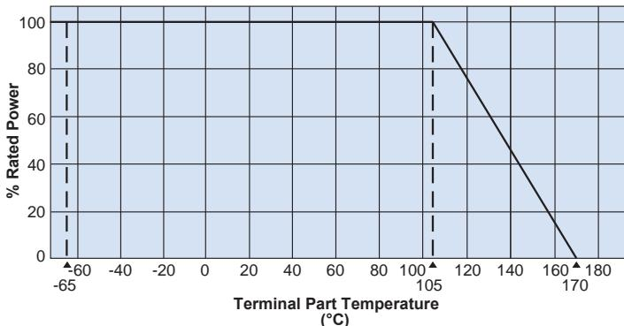
For resistors operated at an ambient temperature of 105°C or above, a power rating shall be derated in accordance with the above derating curve.
