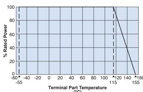
For resistors operated at a terminal part temperature of described for each size or above, the power rating shall be derated in accordance with the derating curve.
