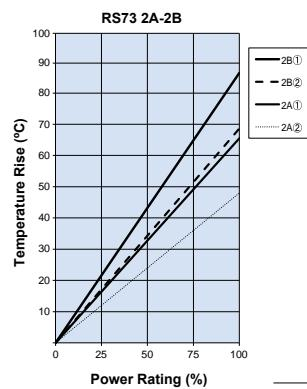
Regarding the temperature rise, the value of the temperature varies per conditions and board for use since the temperature is measured under our measuring conditions.
