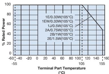
When the terminal part temperature of the resistor exceeds the rated terminal part temperature in the Applications and Ratings chart, the power shall be derated according to the derating curves on the left.
