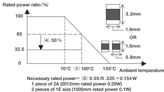
Figure 6. Selection by the traditional derating curve
