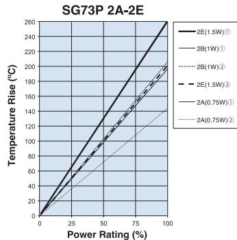
Regarding the temperature rise, the value of the temperature varies per conditions and board for use since the temperature is measured under our measuring conditions.
