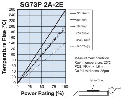
Regarding the temperature rise, the value of the temperature varies per conditions and board for use since the temperature is measured under our measuring conditions.
