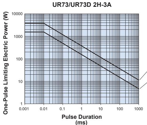
Please ask us about the resistance characteristic of continuous applied pulse. The pulse endurance values are not assured values, so be sure to check the products on actual equipment when you use them.
