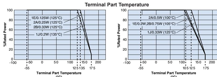
When the terminal part temperature of the resistor exceeds the rated terminal part temperature shown above, the power shall be derated according to the derating curve.
