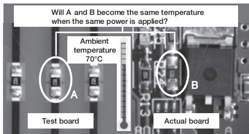
Figure 5. Temperature differs depending on the board
