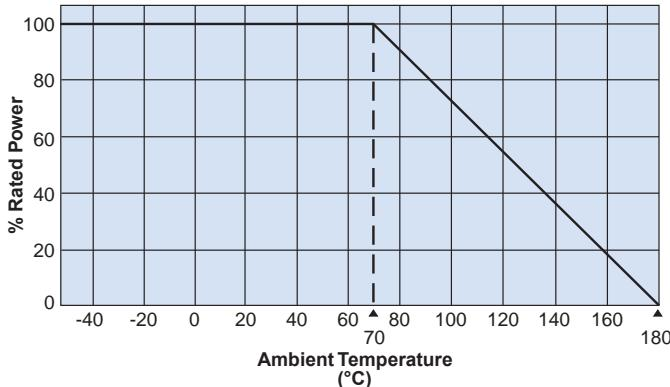
For resistors operated at an ambient temperature of 70°C or above, a power rating shall be derated in accordance with the above derating curve.
