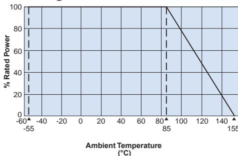
For resistors operated at an ambient temperature of 85°C or above, a power rating shall be derated in accordance with the derating curve.
