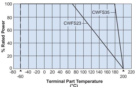
When the rated terminal reference point temperature of the resistor exceeds the rated terminal reference point temperature shown above, the power shall be derated according to the derating curve.
