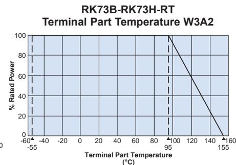
When the terminal part temperature of the resistor exceeds the rated terminal part temperature shown above, the power shall be derated according to the derating curve.
