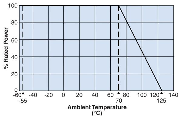
For resistors operated at an ambient temperature of 70 $^{\circ}$ C or above, a power rating shall be derated in accordance with the above derating curve.
