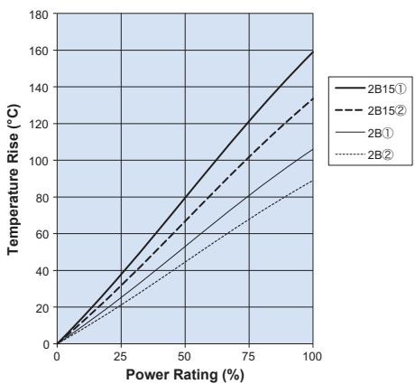
Regarding the temperature rise, the value of the temperature varies per conditions and board for use since the temperature is measured under our measuring conditions.
