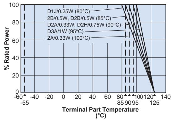
For resistors operated at a terminal part temperature of described for each size or above, a power rating shall be derated in accordance with the derating curve.
