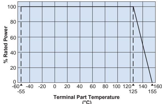
When the terminal part temperature of the resistor exceeds the rated terminal part temperature shown above, the power shall be derated according to the derating curve.
