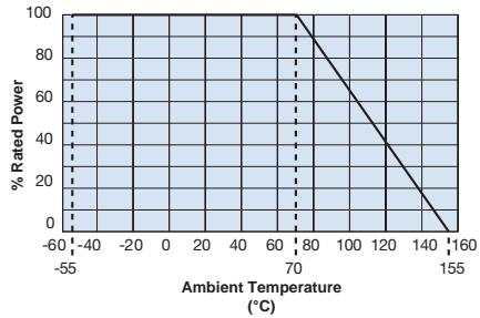
For resistors operated at an ambient temperature of 70°C or above, a power rating shall be derated in accordance with the derating curve.
