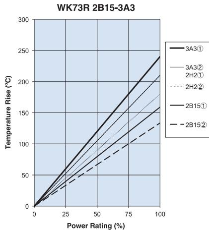
Regarding the temperature rise, the value of the temperature varies per conditions and board for use since the temperature is measured under our measuring conditions.
