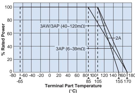
For resistors operated at a terminal part temperature of described for each size or above, a power rating shall be derated in accordance with the derating curve. Please refer to "Introduction of the derating curve based on the terminal part temperature" in the beginning of our catalog before use.
