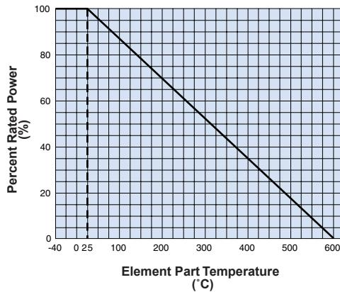
For sensors operated at an element part temperature of 25°C or above, a power rating shall be derated in accordance with the above derating curve.
