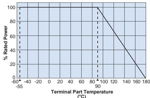
For resistors operated at a terminal part temperature of described for each size or above, a power rating shall be derated in accordance with the derating curve. Please refer to "Introduction of the derating curve based on the terminal part temperature" in the beginning of our catalog before use.
