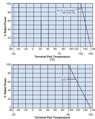
When the terminal part temperature of the resistor exceeds the rated terminal part temperature shown above, the power shall be derated according to the derating curve.
