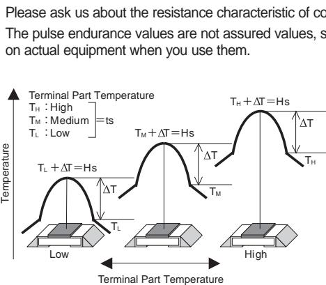
The temperature of the resistor will increase the same  $\Delta T$  from the standard terminal part temperature regardless of the ambient temperature when the same power is applied. This is because there is hardly any heat dissipation from the resistor surface to the ambient air.
