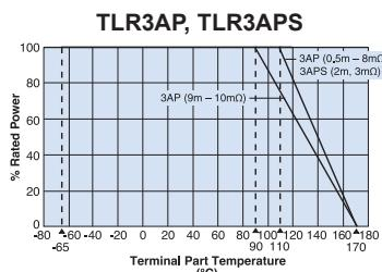
For resistors operated at a terminal part temperature of described for each size or above, a power rating shall be derated in accordance with the derating curve. Please refer to "Introduction of the derating curve based in the terminal part temperature" in the beginning of our catalog before use.
