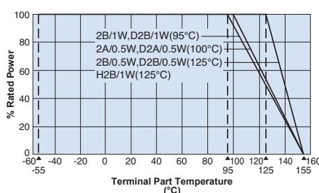
When the terminal part temperature of the resistor exceeds the rated terminal part temperature shown, the power shall be derated according to the derating curve. Please refer to "Introduction of the derating curve based on the terminal part temperature" in the beginning of our catalog prior use.
