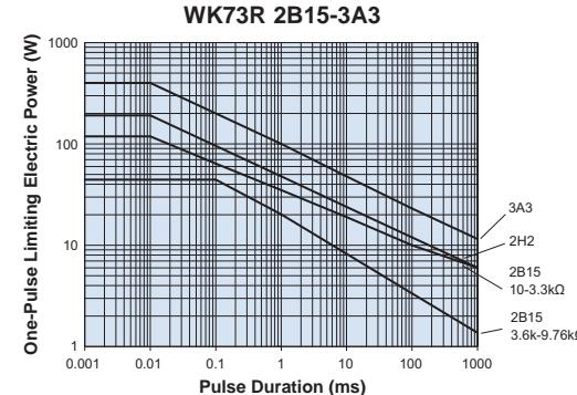
The maximum applicable voltage is equal to the max. overload voltage. Please ask us about the resistance characteristic of continuous applied pulse. The pulse endurance values are not assured values, so be sure to check the products on actual equipment when you use them.
