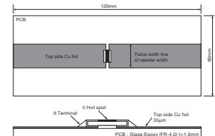
Temperature rise is simulated and measured under our conditions. So, the values will vary depending on the operating conditions and PCB used.
