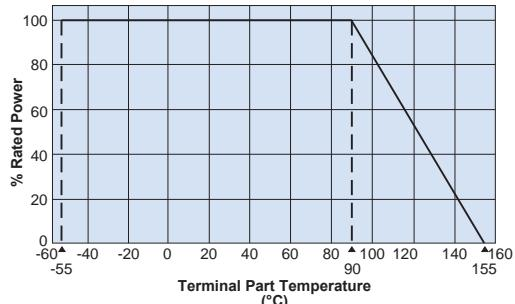
For resistors operated at a terminal part temperature of described for each size or above, a power rating shall be derated in accordance with the derating curve.
