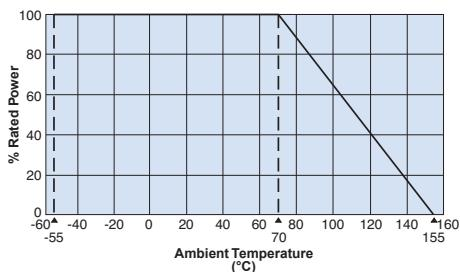
For resistors operated at an ambient temperature of  $70^\circ C$  or above, the power rating shall be derated in accordance with the above derating curve.
