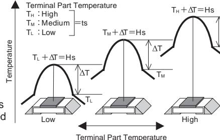
The temperature of the resistor will increase the same  $\Delta T$  from the standard terminal part temperature regardless of the ambient temperature when the same power is applied. This is because there is hardly any heat dissipation from the resistor surface to the ambient air.
