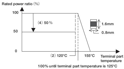
Figure 7. Selection using a terminal-temperature derating curve
