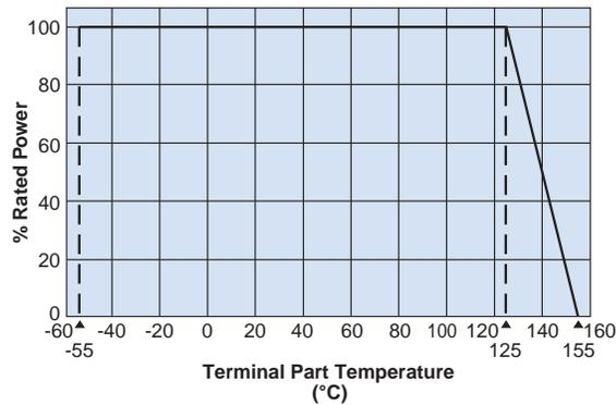
When the terminal part temperature of the resistor exceeds the rated terminal part temperature shown above, the power shall be derated according to the derating curve.
