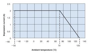
For terminals operated at an ambient temperature of 70°C or higher, the current shall be derated in accordance with the above derated curve.
