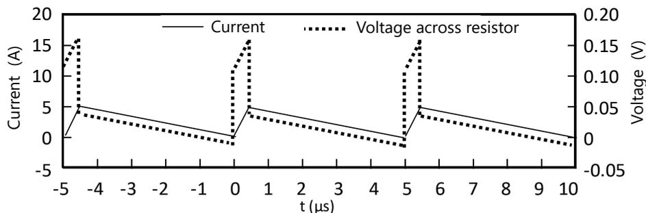
Fig. 11 Voltage waveforms across current sensing resistor
