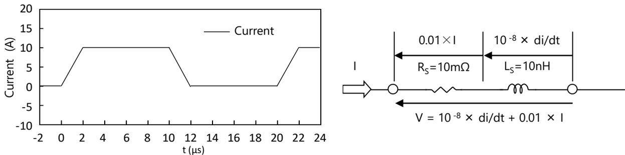
Fig. 5 Linearly changing current waveform and voltage drop
