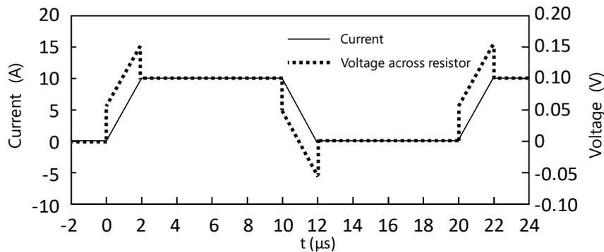
Fig. 8 Voltage waveform across resistor
