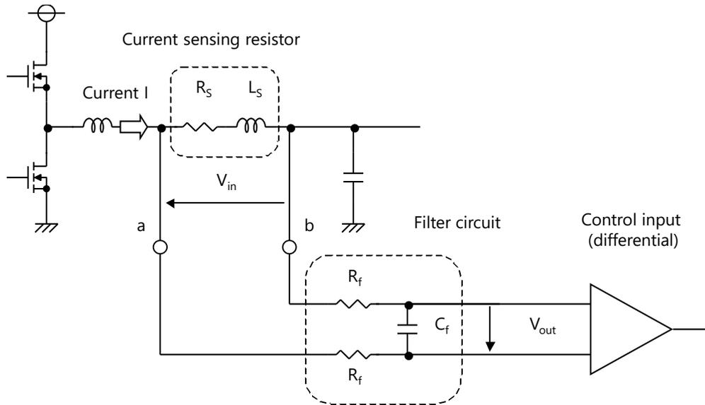
Fig. 15 Filter circuit (differential detection)
