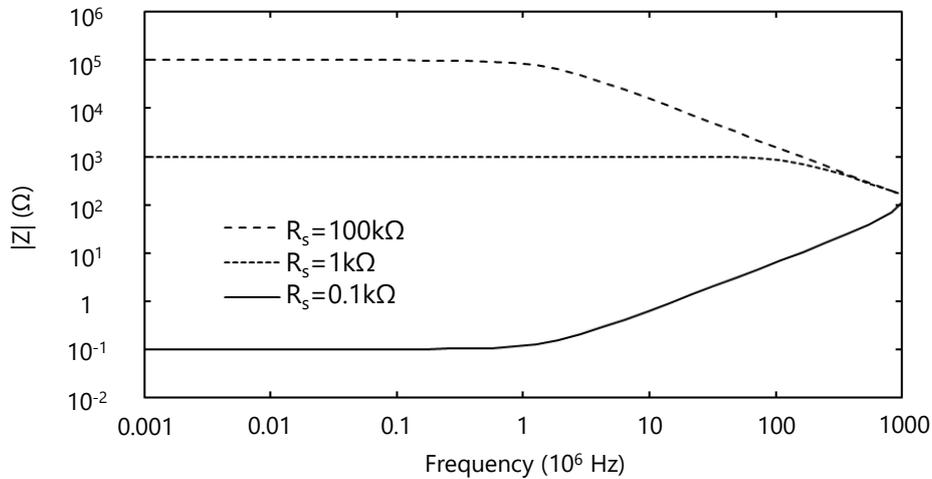
Fig. 2 Effects of  $R_s$  on frequency characteristics of impedance  $|Z|$
