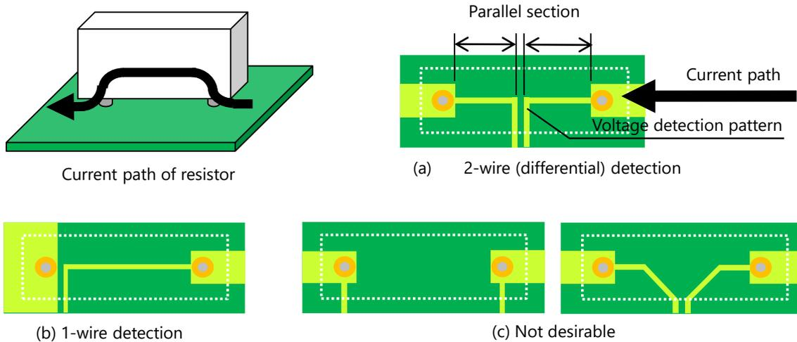
Fig. 13 Example of voltage detection pattern of leaded resistors
