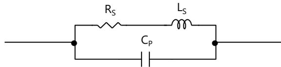
Fig. 1 Equivalent circuit of resistor
