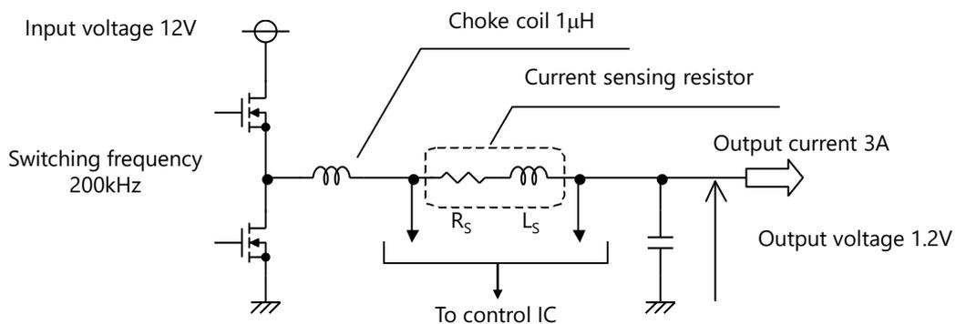
Fig. 9 DC-DC converter output circuit
