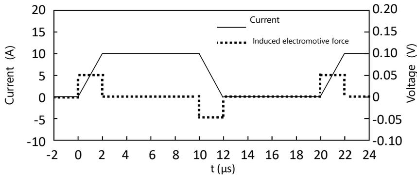
Fig. 7 Induced electromotive force caused by  $L_s \times di/dt$
