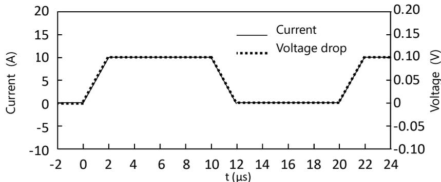
Fig. 6 Voltage drop caused by  $R_S$  and current
