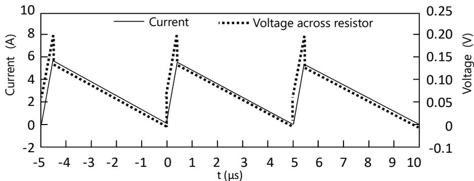
Fig. 12 Voltage across current sensing resistor when  $R_S = 50\text{m}\Omega$
