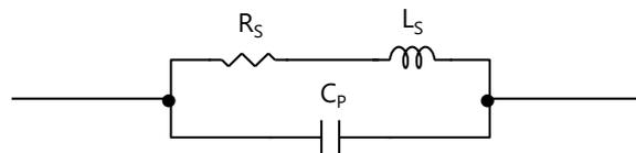
Fig. 1 Equivalent circuit of resistor
