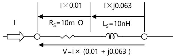
Fig. 4 Voltage drop at 1MHz of 10mΩ resistor
