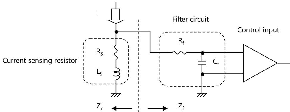
Fig. 16 Filter circuit (one-wire detection)
