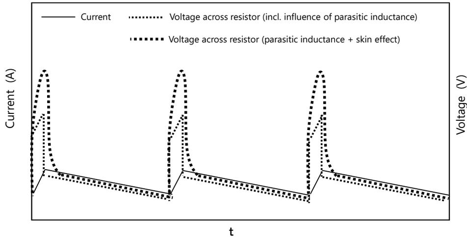
Fig. 18 Current sensing waveform of DC-DC converter output under the influence of skin effect
