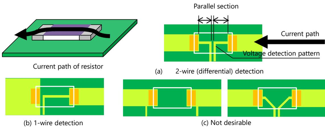
Fig. 14 Example of voltage detection pattern of surface mount resistors
