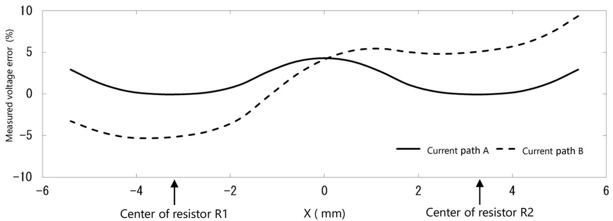
Fig. 4 Changes in measured voltage error effected by current path and voltage measuring position
