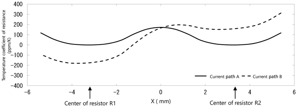
Fig. 5 Changes in T.C.R. effected by current path and voltage measuring position.
