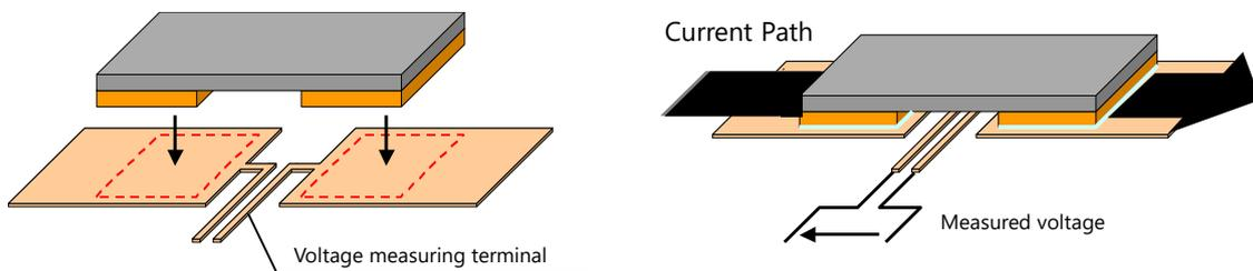
Fig.1 Recommended current path and voltage measurement position when using a single resistor.
