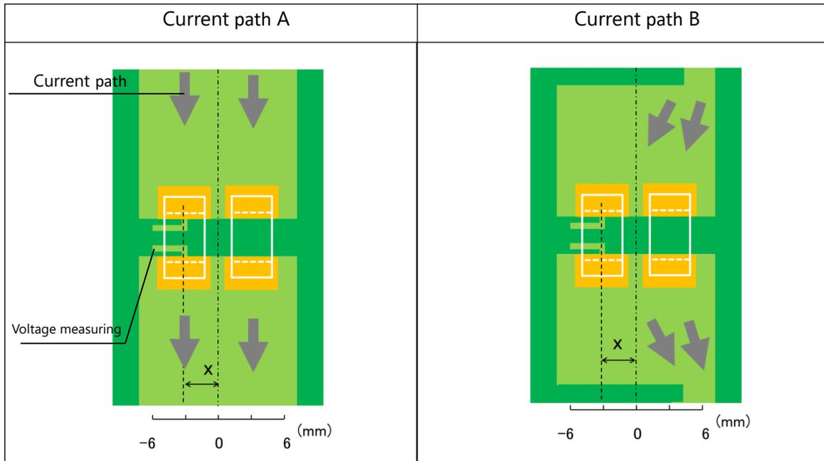
Fig. 3 Voltage measuring position
