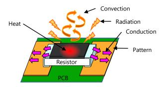
Fig.10 Image of heat generation and heat release of resistor
