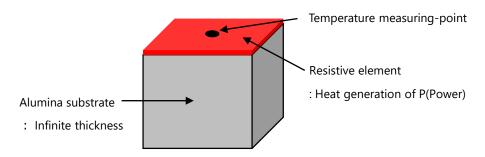
Fig.11 Simplified model for confirmation of temperature rise
