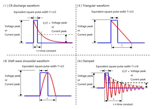
Fig.6 Methods of conversion to equivalent square waves
