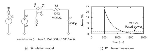
Fig.1 Simulation of pre-charge circuit
