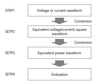
Fig.5 Evaluation procedure of pulse power capability
