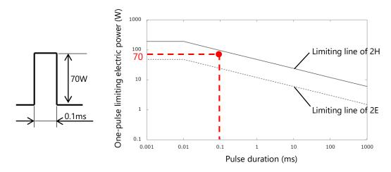
Fig.9 Example of evaluation using one-pulse limiting electric power of thick film chip resistor (RK73B)
