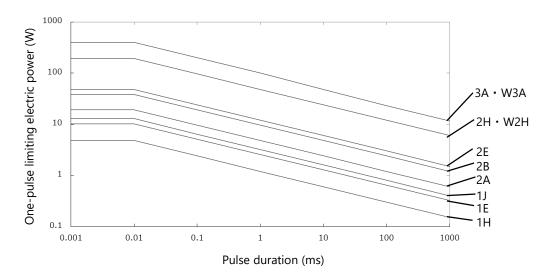
Fig.4 One-pulse limiting electric power of RK73B
