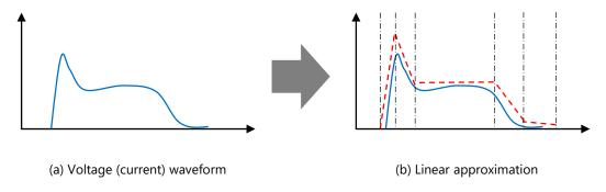
Fig.7 Linear approximation of pulse waveform
