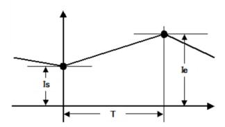
Fig.8 Calculation of energy by interval integration (with current)
