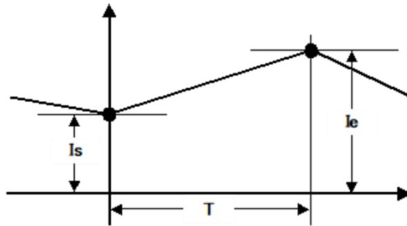
Fig.8 Calculation of energy by interval integration (with current)
