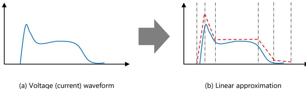
Fig.7 Linear approximation of pulse waveform
