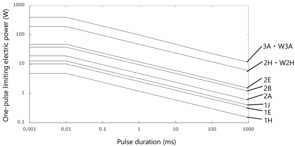
Fig.4 One-pulse limiting electric power of RK73B
