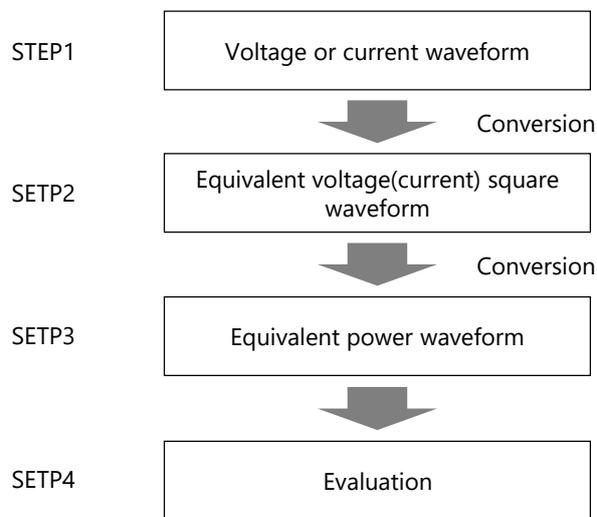
Fig.5 Evaluation procedure of pulse power capability
