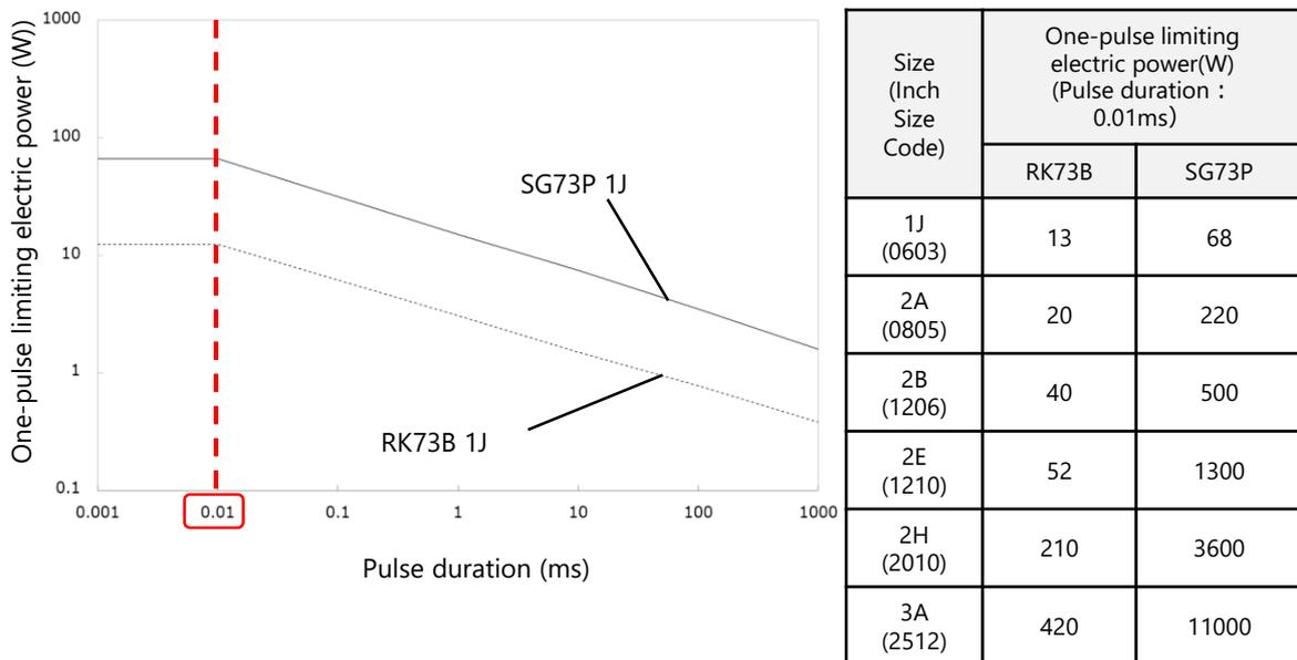
Fig.14 One-pulse limiting electric powers by type and size of resistors
