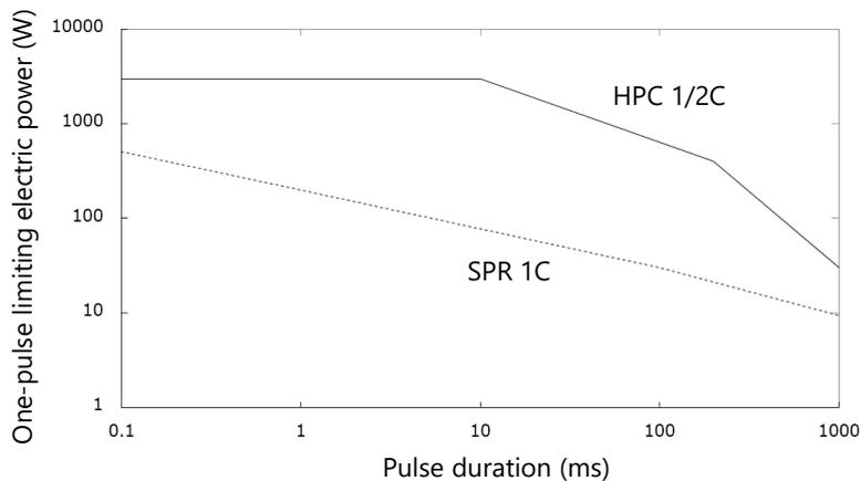
Fig.2 One-pulse limiting electric power diagram of HPC 1/2C and SPR 1C
