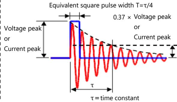
Fig.6 Methods of conversion to equivalent square waves
