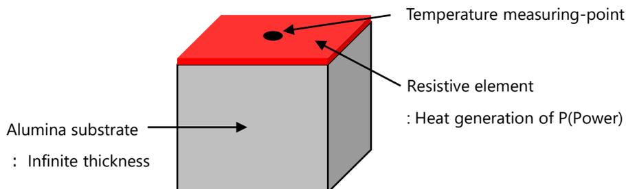
Fig.11 Simplified model for confirmation of temperature rise
